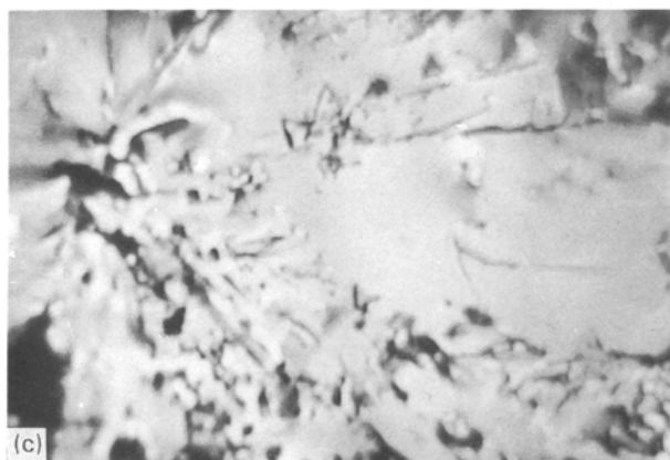
Figure 6 Surface appearances and crystallization from a \text{Bi}_{1.9}\text{Sb}_{0.1}\text{Sr}_2\text{Ca}_2\text{Cu}_3\text{O}_8 composition melt, as observed by a thermo-microscopic apparatus: cooling to (a) 812 °C and (b,c) 802 °C. The horizontal dimension of each print corresponds to 300 \mu\text{m} .
